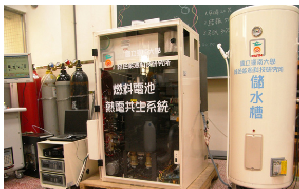
Fig. 5. Photo of the present fuel cell cogeneration system.
